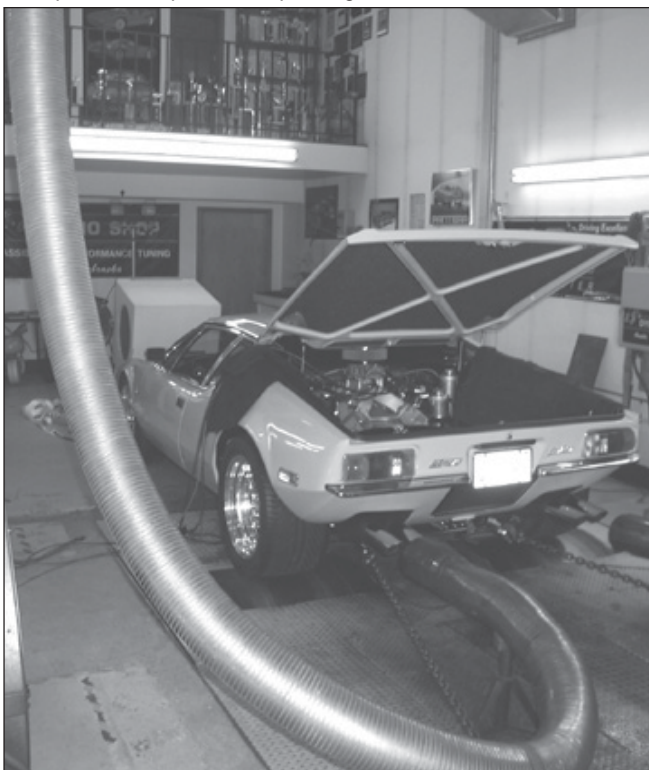
Above: The cylinder block is a Dart brand. Crane cam actuates Jesel 1.6 rockers. Heads are the powerhouse Yates aluminum C3L models. Below: E.J. Poss' dyno separates fact from fiction. 500 plus horsepower is the proof of the pudding.
