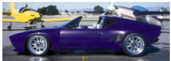
Above: The Gary Hall car has 17 inch wheels. This car obviously uses a higher front rake of about 1 inch. Any rake should be the opposite, with a lower front. As we see on the picture, the top part of the tire hides in to the wheel well. An impossible
