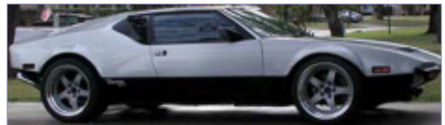
Above: Kirby Schrader's new 18-inch Kinesis wheels. The front wheels were delivered with 1/2 "too much + offset. Together, with the bigger diameter tires, the car ended up very high.
